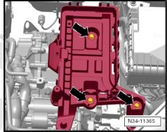
Remove securing clip in -direction of arrow-.
