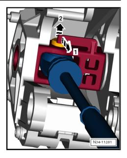
Please insert -screwdriver- from underneath whilst pushing securing tab forwards.
