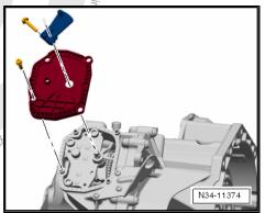
Working through opening, push selector fork to side -direction of arrow-.
