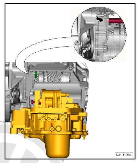
The "sticking" gear actuator -a its "removal position". To do the parking lock cover. How to do work procedure:
