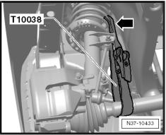
Remove right flange shaft of gearbox.
