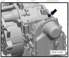
Attach all retainers and brackets to front of gearbox.
