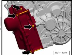
Make sure that plungers meet up correctly in cups of engaging levers.
