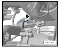
Use your hand to press lever to stop in direction of cable support bracket.
