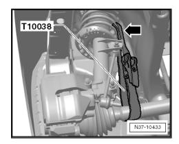
Remove right flange shaft of gearbox.
