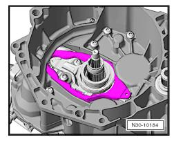
Remove bolts and remove small engaging lever.
