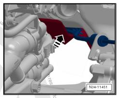
Loosen adjustment screw -arrow-.
