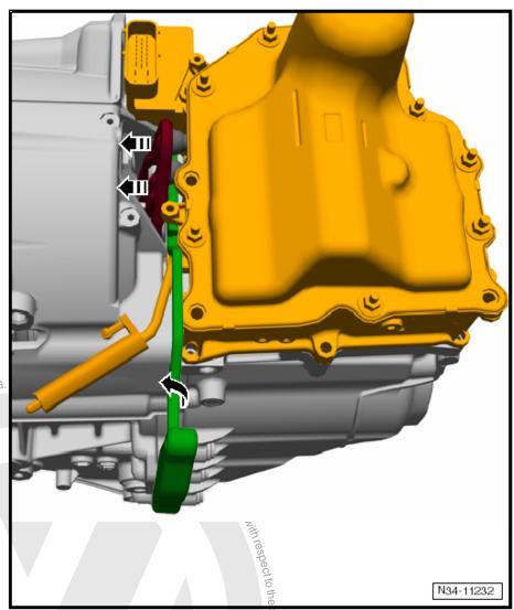
Do not take out assembly lever between engaging lever and goess.
