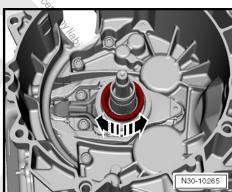
Secure shim using 3 drops of glue -AMV 195 KD1 01- .
