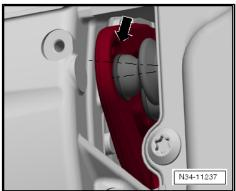
Turn assembly lever -T10407- clockwise and remove it.
