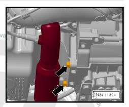
Support engine and gearbox with support bracket -10-222 Abut do not raise.
