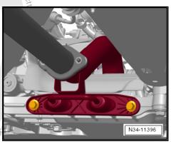
Remove front exhaust pipe so that lower bolts can be removed -arrows-. . DA nagewagen AG.
