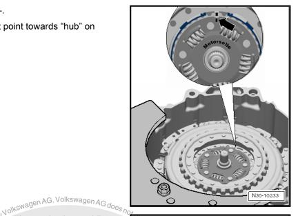
Turn clutch by hand and observe "Small" engaging lever whilst turning.
