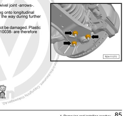
Secure both drive shafts to suspension struts using tensioning straps -T10038-.
