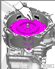
Engaging levers must remain "still" in their position whilst this is being done. They are not allowed to move up and down.
