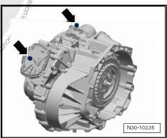
Secure gearbox on gearbox support -VW 353-
