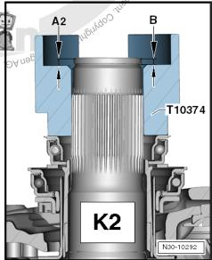
Install parts of clutch as far as large engaging lever
