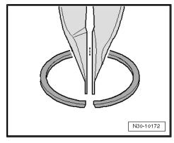
If you can insert retaining ring -arrow-, clutch is correctly pressed on to stop.
