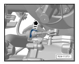
Remove -selector housing- beneath selector lever.
