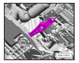
Support engine and gearbox with support bracket -10-222 Abut do not raise.
