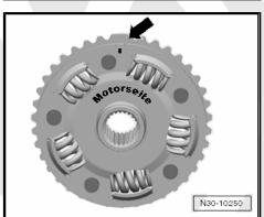
"Large" tooth has a mark on -engine end- -arrow-.
