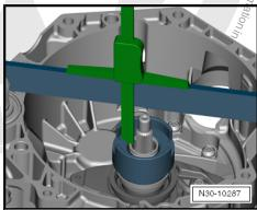
Measure distance from "shaft end" into gauge block -T10374-.
