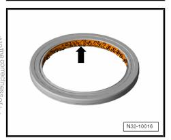
Drive in new seal to stop, being careful not to cant seal.
