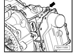
Remove all retainers and brackets from front of gearbox.
