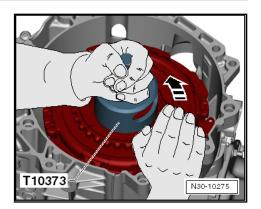
In this way, clutch slides against retaining ring. Do not use any other tool.
